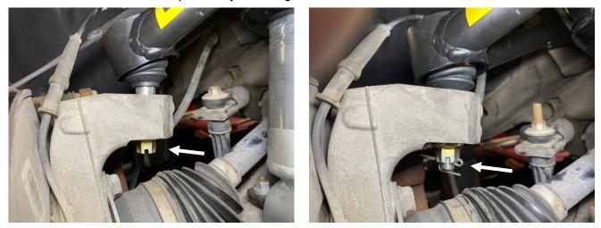
R. Using the supplied hose clamp, screw, locknut, and 2 washers, secure the ABS line to the tab on the UCA as shown below. Using a 3/8 wrench and 1/8" allen, tighten the screw and nut, then verify ABS line has adequate slack to accommodate steering and suspension motion.
