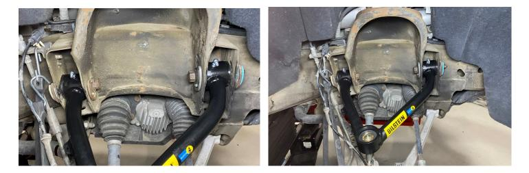
O. Reinstall the shock and spring assembly. Secure 3 top mount nuts using an 18mm wrench and lower mount using 15mm wrench and socket. Reattach the wiring harness clips to the top mount studs. Then reinstall the stabilizer link using a 15mm wrench and socket. Torque all hardware to OE specifications according to the manufacturer service manual.
