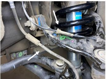
D. Using a 10mm socket, remove the ABS bracket from the top of the spindle and disconnect the ABS line from the plastic clip.
